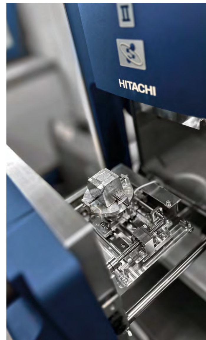
The sample stage is pulled completely out of the chamber for easy sample changes
