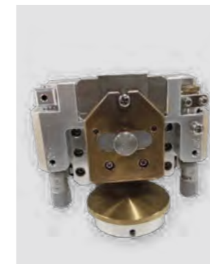
Cross-section holder for large samples Up to 35mm width, 17mm depth, 8mm height
