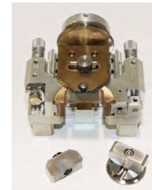
Cross-section set Preparation of cross sections
