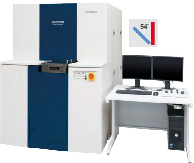
NX2000 is a FIB-SEM optimised for semiconductor applications (defect analysis with KLARF coordinate import, TEM lamella extraction, device development). With 205 x 205 mm X,Y travel, the sample stage even allows full-surface processing of 200 mm wafers without sample rotation. The vertically mounted Ga FIB allows up to 100nA ion current at 30 kV. The FE-SEM column is equipped with a cold field emitter.
