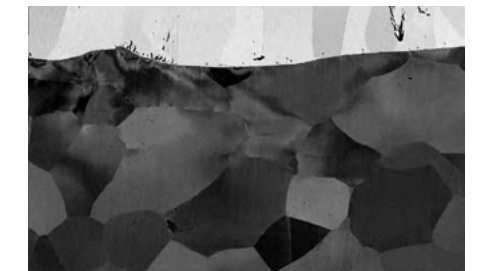
Zinc coating on steel
