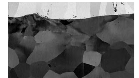
Zinc coating on steel
