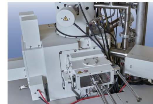
The specimen exchange chamber accepts large specimens up to  $\Phi 150$  mm diameter. Multiple EDS ports in the improved chamber design offer versatile analytical platform. (The instrument picture includes options)
