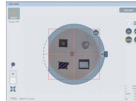
The built-in optical camera captures the specimen holder overview and is automatically transferred to the SEM MAP screen for a graphical navigation interface to assist with quick access ROI.
