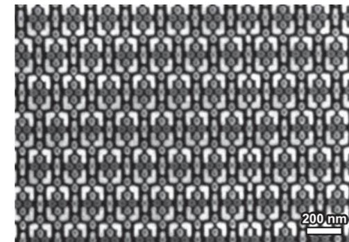
Voltage contrast in a SEM is a very powerful tool for semiconductor device evaluation. As the device structure changes by layer, SEM conditions such as accelerating voltage and contrast must also be optimized. The SU8700 offers a voltage range down to 0.1 kV, without stage bias, to address these needs and more. On the left is an image taken at 300 V to demonstrate this VC capability as applied to the analysis of device architecture.
