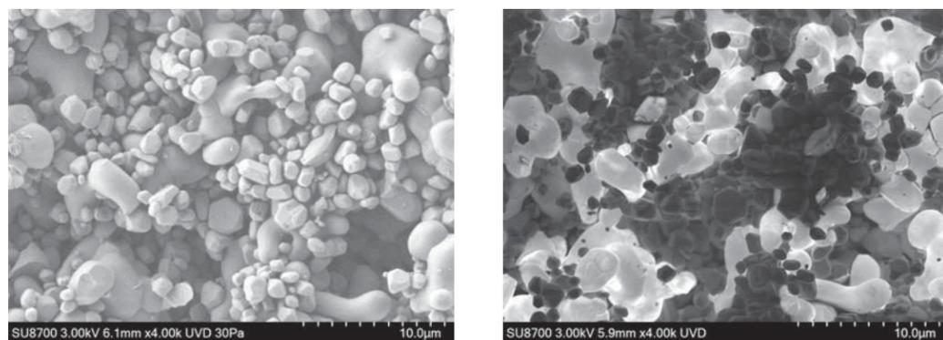
The SU8700's unique UVD collects photonic signals in order to provide information beyond traditional EM methods. The left image demonstrates the UVD being used as a variable-pressure SE detector which in order to display surface and morphological information of this specimen. Whereas the right image demonstrates the UVD operating as a Cathodoluminescence detector under high vacuum conditions to clearly show the distribution of the fluorescent pigments.
