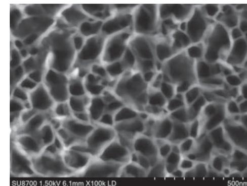
The ability to visualize high-quality topographical information is an essential capability for all modern SEM platforms. The SU8700 LD enables acquisition of topographical information with outstanding detail, speed, and definition. The image left on the left reveals surface topographical information of anodized aluminum oxide.
