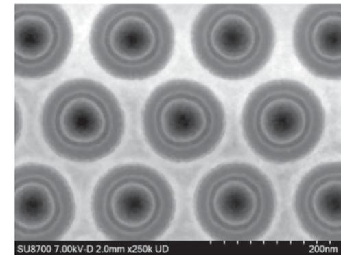
The image on the left shows analysis of memory cell structure for 3D NAND. This data clearly shows structure consisting of very thin (<10 nm) nitride, oxide and poly-Si layers. The high detection efficiency of the SU8700 allows for precise analysis of such features which are crucial to understanding capacitor structure.
