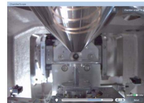
GUI integrated chamber scope provides safe operation by showing specimen position in real-time. Monochrome/color convertible and can be displayed on individual window.
