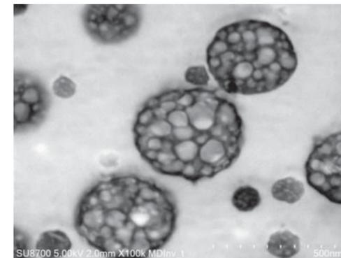
Backscatter electron (BSE) imaging is a powerful tool for acquiring compositional information of specimens. The image on the left shows a Salami structure stabilized by stained ABS resin with the SU8700's MD. The SU8700's MD allows for TEM-like data acquisition and even works at voltages lower than 0.5 kV.
