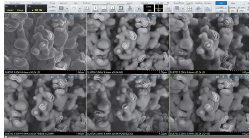
Multi-Channel image can be displayed on the screen. 2, 4 or 6 signals including the chamber scope(\*) or SEM MAP image can be displayed simultaneously on a single monitor. (top)
