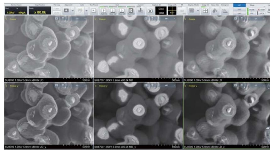
In multi-signal display mode, a saved image can be loaded to a vacant channel and further processed for real-time comparison to live conditions. (bottom)
