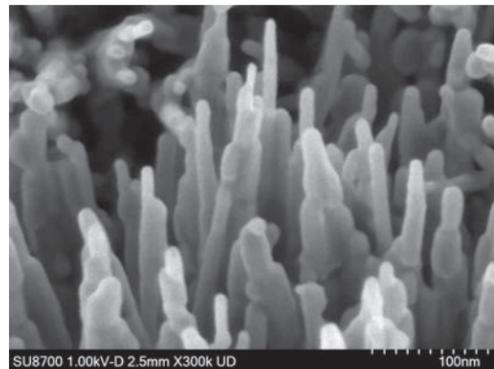
The new UD is well-suited for fine structure imaging by utilizing superior low-energy signal collection. The image above shows nano-scale morphological information of needle-like TiO<sub>2</sub> with tip radii of less than 10 nm.
