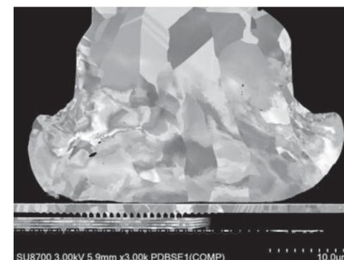
An essential capability of a BSE detector is the ability to acquire crystallographic as well as compositional information. The image on the left shows bonded gold wire's grains, voids and deformation at 3 kV to clearly demonstrate the PD-BSED's high sensitivity and ability to distinguish between structural components.
