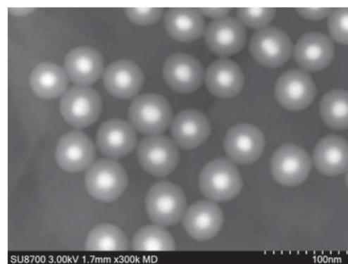
Many modern nanoparticles contain a core-shell design that is vital to their functionality. It is essential to measure size of both the core and the shell in morphological evaluation as well as functional characterization. In the left image above, fine surface structure is visible by SE signal (UD). In the Right image, Core (Ag) and Shell (SiO<sub>2</sub>) are easily distinguishable by BSE signal (MD).
