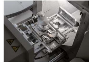
Right: external view of the stage. XY movable range: 135 x 100 mm
