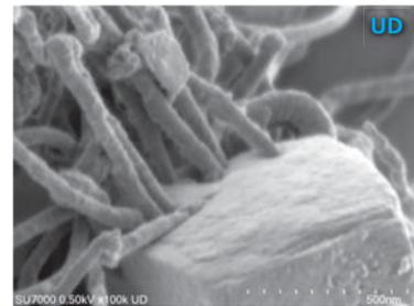
Evaporated metal particle with CNT composite material
