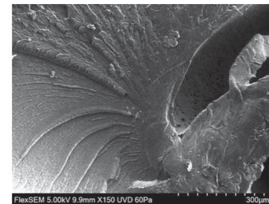
FlexSEM 5.00kV 9.9mm X150 UVD 60Pa Accelerating voltage: 5.0 kV, Magnification: 150x Signal: UVD-II Specimen: resin fracture
