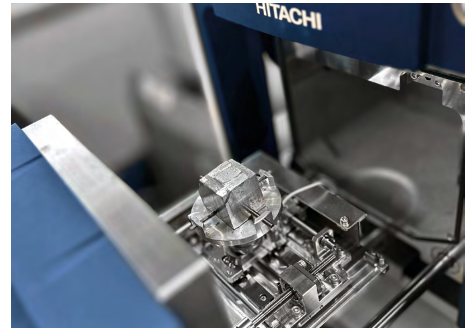
The specimen stage withdraws completely from the chamber for easy sample changes
