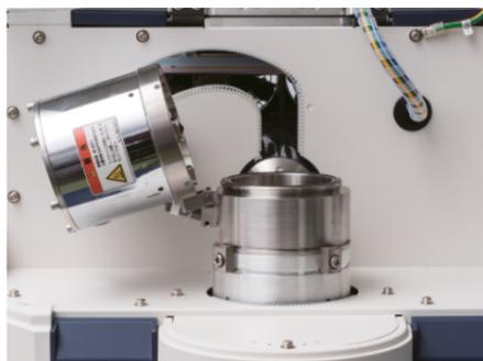
Figure 3. FlexSEM's electron gun flipped open for direct access to the filament cartridge.
