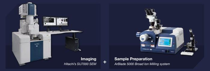
Combining the imaging power of **Hitachi's SU7000 SEM** with the sample preparation capabilities of the **ArBlade 5000 Broad Ion Milling system** made particularly challenging preparatory tasks solvable. Components from the pacemaker industry could be easily prepared and sectioned, which would have been difficult with other technologies under consideration by the company.
