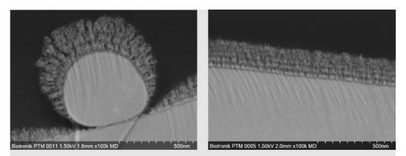
The cross section with the ArBlade 5000 using the metal-primer-resin system reveals a gap-free and perfect bond between the materials involved.
