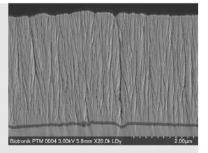
The cross section with the ArBlade 5000 by the metal adhesion layer functional layer system reveals a thin adhesion layer in the range of 80nm to 90nm.
