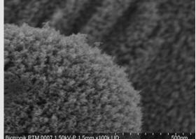
At high magnifications, a nanostructure becomes visible on the surface that has not been observed before and is subsequently mainly responsible for the adhesive properties and the absorption of the primer.
